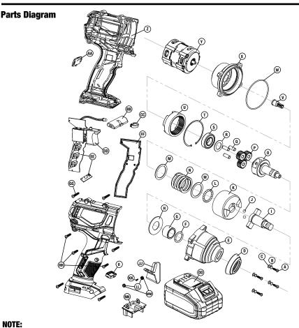
Not all components of the Impact Wrench are replacement items, but are illustrated as a convenient reference for location and position in the assembly sequence.
