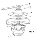
**NOTE:** If the clamp nut cannot be loosened by hand, use the wrench (3) provided. DO NOT remove the disc flange (4).
