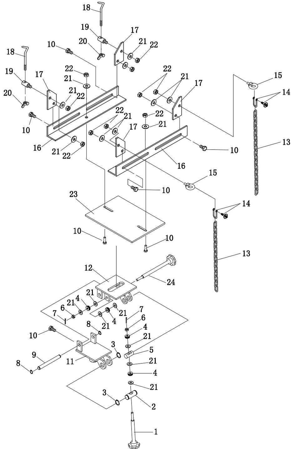
**NOTE:** Not all components of the Transmission Jack are replacement items, but are illustrated as a convenient reference for location and position in the assembly sequence.
